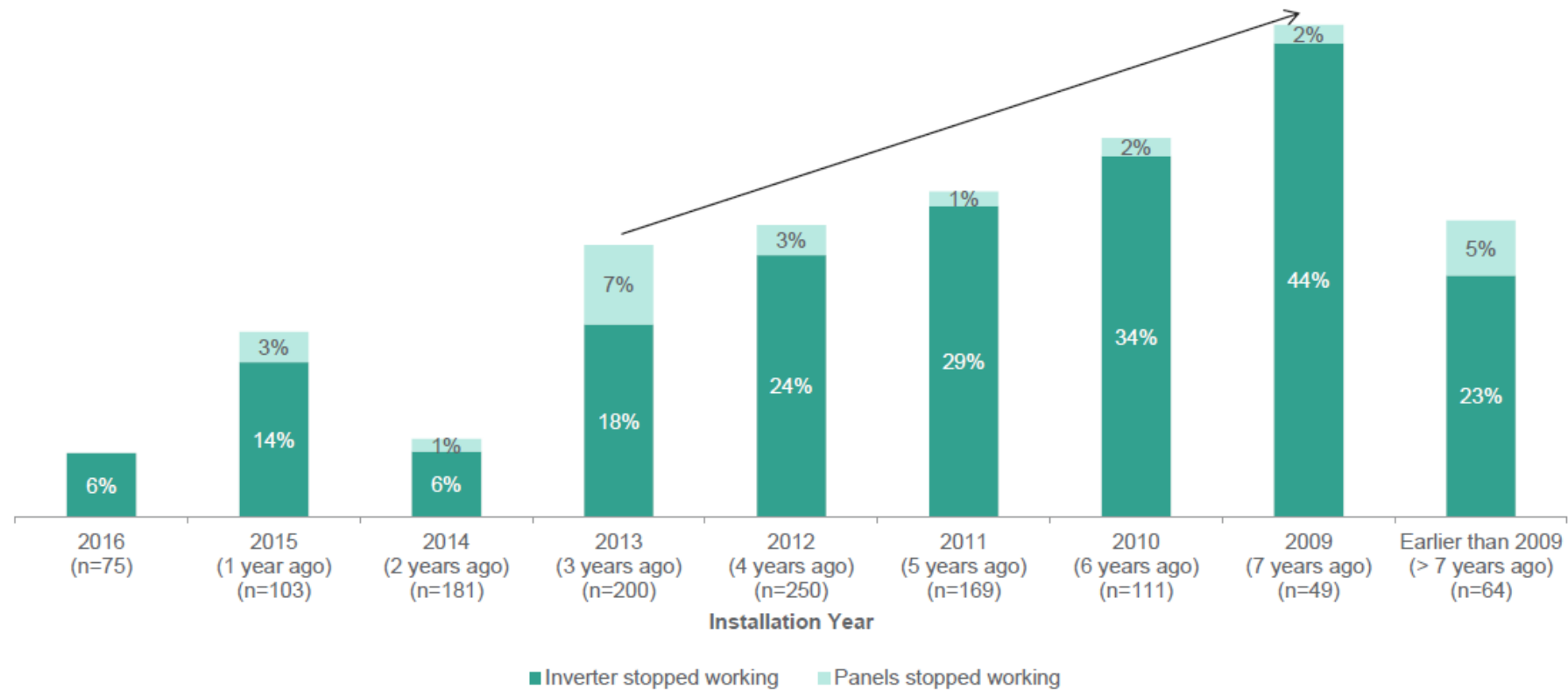
Issues Experienced With Solar PV Systems
